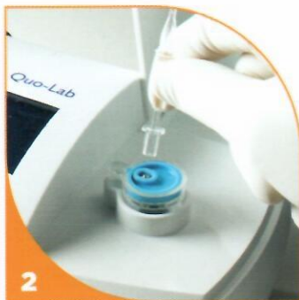
2 When prompted press reagent bead into cartridge using the reverse end of the sampling tool.
