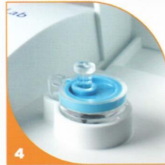
4 Close analyser lid. Result displayed within 4 minutes.
